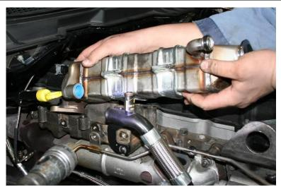
15. Remove the cooler mount bolts to the head (13mm socket) and remove the cooler mount from the vehicle.
