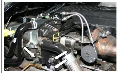
6. Remove the three bolts for the stepper motor bracket (10 mm) socket and prop the bracket on the cooler.
