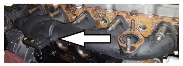
Please note the M12 inverted flare port is for the OEM back pressure sensor.
