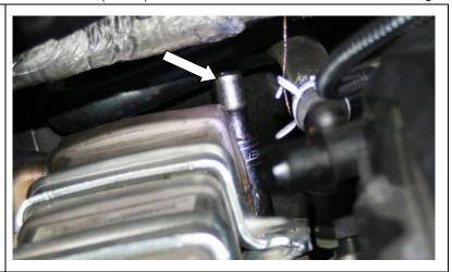
14. Prop the cooler above the studs and push towards the cab holding the other coolant hose to release the oring fitting to remove the cooler from the vehicle.
