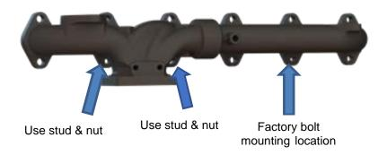
3. The five exhaust manifold cap screws with studs are used at the No. 1 and No. 2 cylinder locations for the heat shield mounting and one on the rear lower corner of the manifold for the cabin heater tube bracket.
