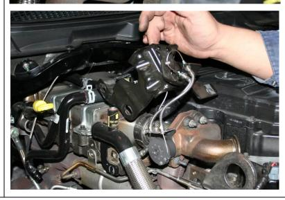
7. Loosen the clamp (11mm) that connects the EGR Flow Direction Valve to the cooler and slide the clamp towards the valve.
