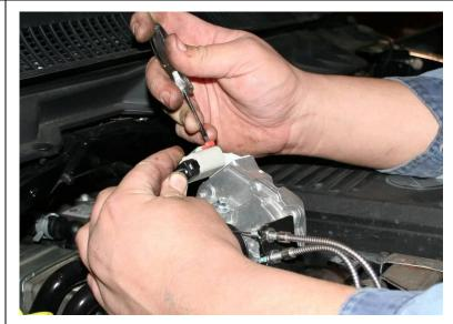
2. Next unplug the stepper (servo) motor connector and remove the two bolts (8mm) that hold the motor to the stepper motor bracket. Then release the cable to remove the motor from the vehicle.
