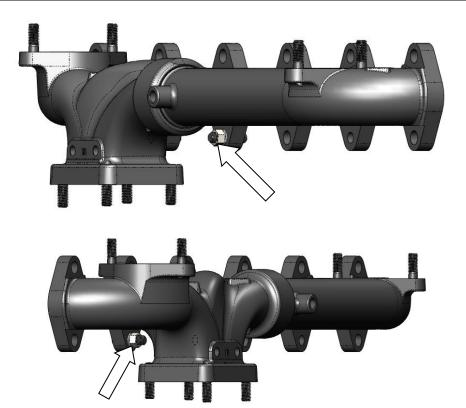
Arrows point to the locations of 30mm studs. All 25mm studs are installed in the EGR ports and T4 flange.
